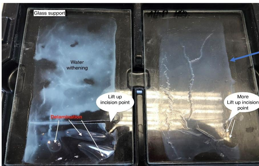
Crack bridging tests > class A5
